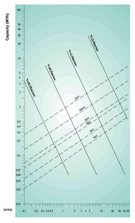
Loss of head (meters) for 100 meters multygol pipe
